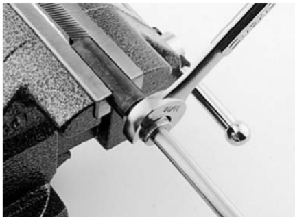
Place Pre-Setting Tool in a vice and tighten nut specified number of turns.
